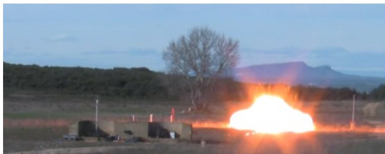
Figure 2. Propane vapor cloud explosion tests
