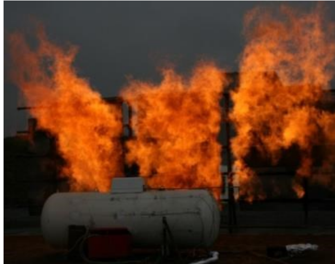
Figure 3. Gas fueled burning wall impacting an LPG tank
