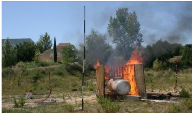
Figure 1. Test of wooden fence fire on LPG tanks
